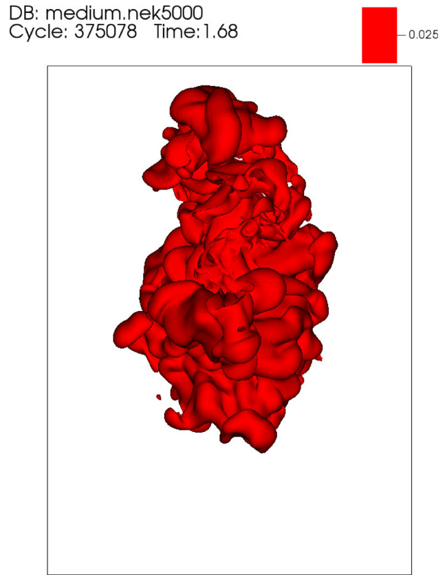
FIG. 10. Video 3: Front y - z view showing the temporal evolution of the \theta = 0.025 isosurface for the DNS of a mild cough. Time is in seconds. Multimedia view: http://dx.doi.org/10.1063/5.0042086.3
