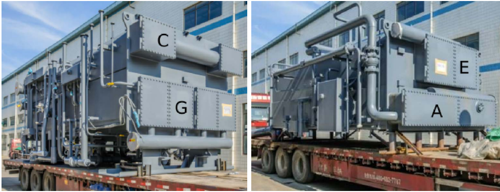
Figure 17: Current heat transformer: Ebara, nominal capacity \approx 7 MW, A: Absorber, G: Generator, E: Evaporator, C: Condenser (All Rights Reserved, Copyright Ebara Refrigeration Equipment & Systems Co., Ltd. 2019)
