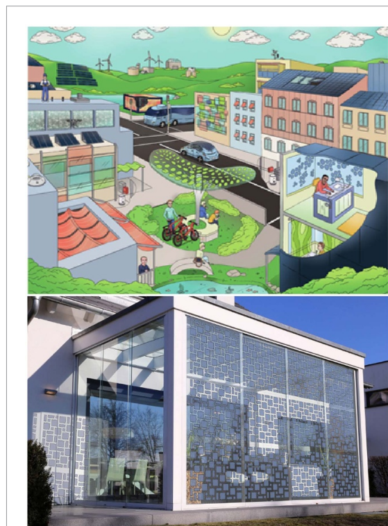
Figure 4. Top: visionary concept of the OPV product portfolio. Flexible, colourful and semi-transparent modules are integrated indoors as well as outdoors into windows, facades, installations, green houses, urban mobility concepts or mobile applications and are becoming part of the daily life, making renewable energies available ubiquitously. Bottom: 'Real World' integration of OPV modules in glass construction elements. Reproduced with permission. (Courtesy Armor SPF GmbH).
