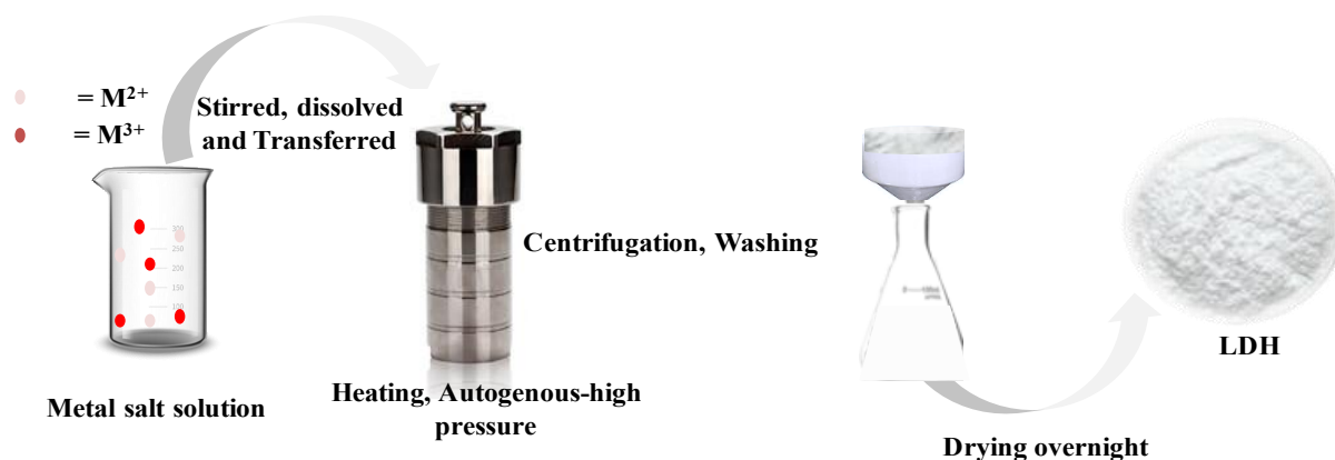
Fig.4. Schematic representation of the synthesis hydrothermal process of LDH.
