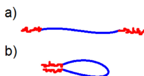
Figure 1. Two distinct conformations of telechelic unimers: (a) hydrophobic blocks (red) are separated and (b) hydrophobic blocks are reversibly connected, and the hydrophilic block (blue) forms a loop.
