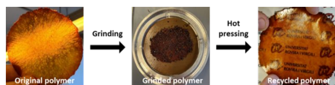
Figure 6. Photographs of the original, grinded and recycled samples of the poly(acylhydrazone)s.
