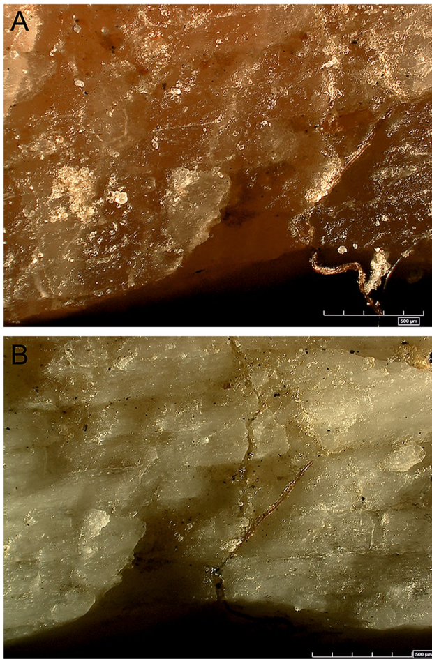
Fig. 5 A Experimental sample (08–20.4) before cleaning with acetone. B Same control point of the sample after cleaning (stage 3). After the cleaning, the greasy appearance remained. Some of the tissues and residues remained on the surface. Images obtained with a 3D digital microscope with lateral source of light. Original magnification: 140 \times . Scale bar: 500 \mu m
