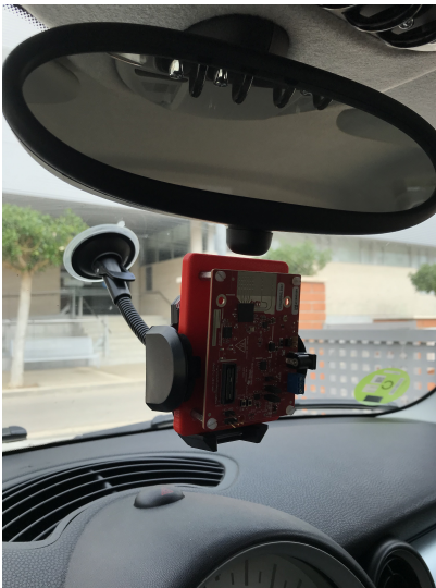
Fig. 4. Photograph of the radar attached to the front glass for testing.
