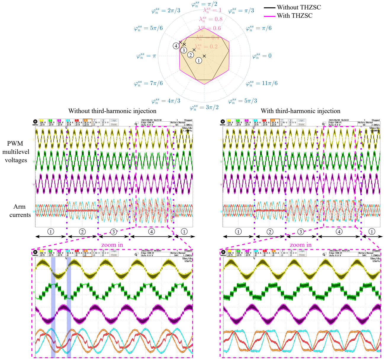
Fig. 8. Experimental waveforms for different negative-sequence current injections corresponding to ①, ②, ③, ④, for balanced grid voltages, and \lambda_{pq}^{ss} = -0.5 . Left column: Without optimal THZSC injection. Right column: With optimal THZSC injection. Channels CH1, 2, and 3 show the PWM converter voltages v_x , and Channels CH4, 5, and 6 show the arm currents i_{arm-x} .
