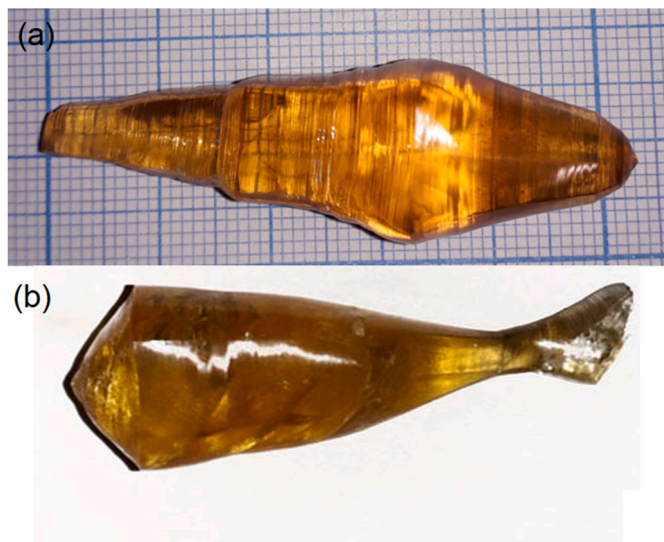
Fig. 2. Photographs of the as-grown crystal boules of (a) undoped \text{MgMoO}_4 and (b) 0.1 at.% \text{Tm}^{3+} -doped \text{MgMoO}_4 (actual doping level). The growth direction is along the [001] axis.
