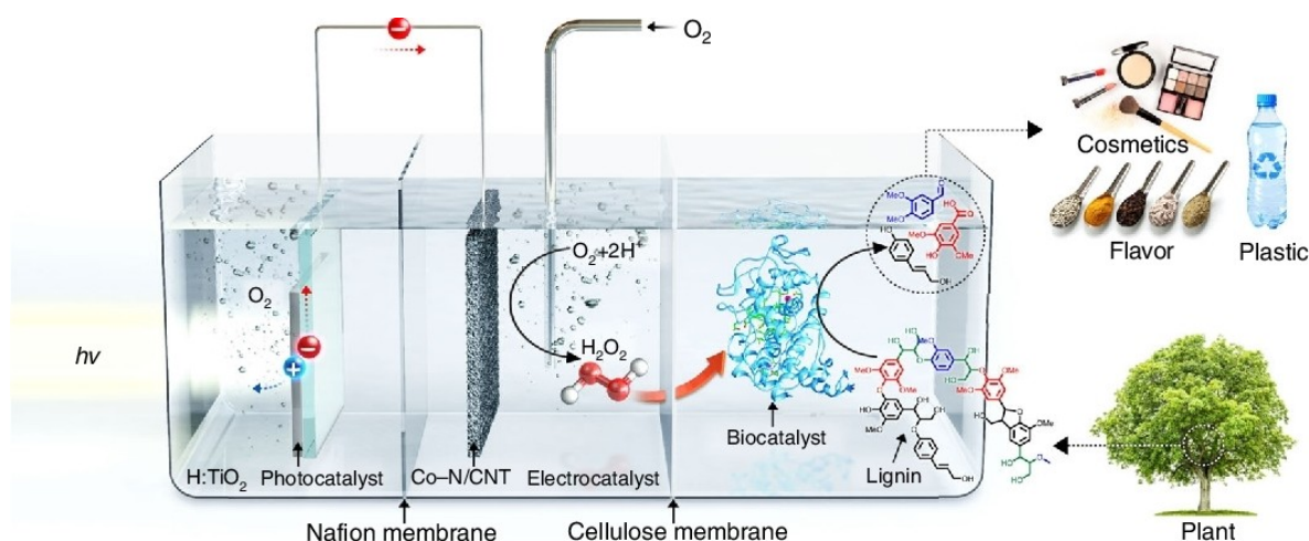
Figure 2. Coupled three-compartment photo-electro-biochemical reactor for lignin depolymerization [Reprinted with copyright obtained from ref. [52]].
