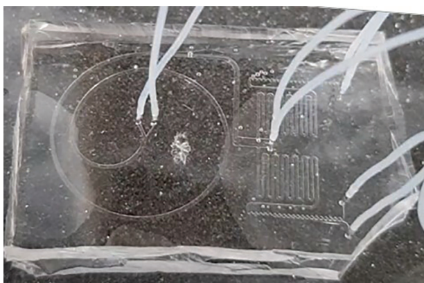
Figure 3. Final device fabricated, consisting of a separator connected to mixers and concentrators.
