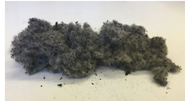
Fig. 2 Polyester mat of recycled fiber from tire
