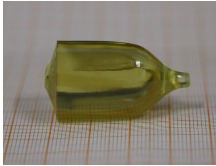
Figure 1. A photograph of an as-grown Yb, Ho, Eu:CNNG crystal (11.5 at.% \text{Yb}^{3+} , 1.25 at.% \text{Ho}^{3+} , 0.075 at.% \text{Eu}^{3+} ), the growth direction is along the [111] axis.
