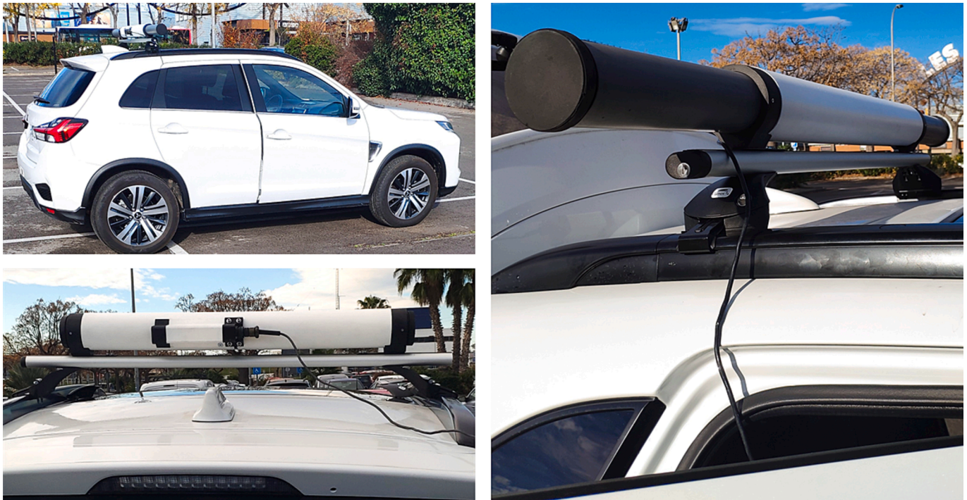
Fig. 2. Mobile unit with two \text{LaBr}_3(\text{Ce}) in a retractable platform coupled on the car roof developed by URV.
