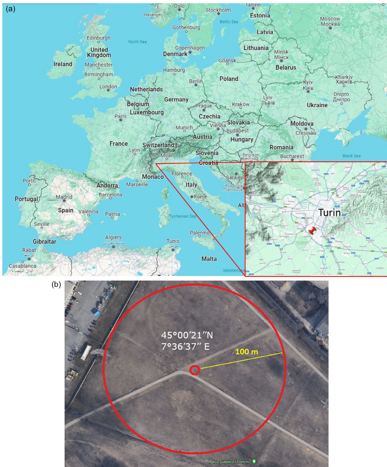
FIGURE 1 (a) Google Maps picture identifying the location of the site selected for the reference station. (b) Google Earth picture of the site, with the 100 m radius free of obstacles around the station, positioned in the centre of the red circle. The coordinates of the station are reported in the picture. It is worth mentioning that all trees have been cut in the area internal to the red circle, according to the WMO prescriptions, in order to reduce uncertainties in the data representativeness and measurement errors. [Colour figure can be viewed at wileyonlinelibrary.com ]
