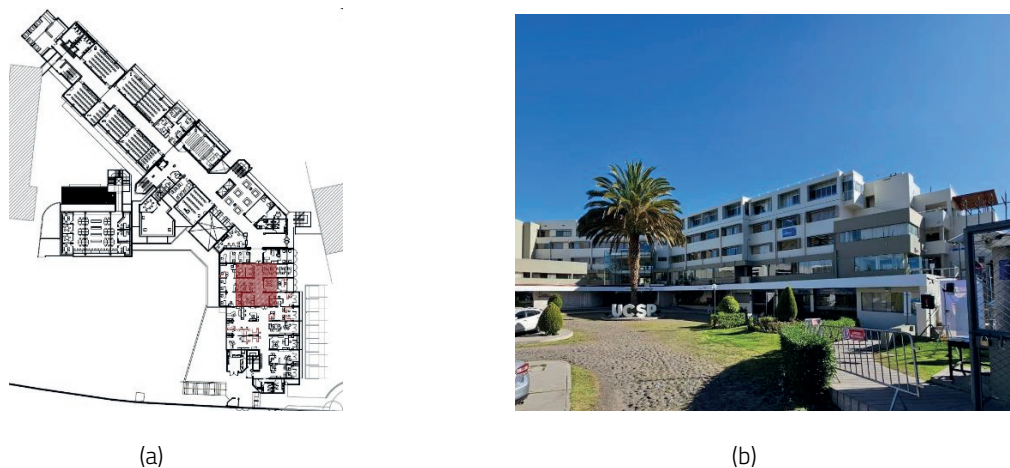
Figure 2. UCSP St. John H. Newman Building, (a) Plan of the building with the office spaces without ventilation or natural lighting marked. (b) photo of the facade of the building. Own elaboration.
