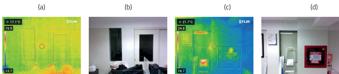
Figure 4. (a) (b) Thermographic photograph 1 of the exterior of room N202; (c) (d) Thermographic photograph 2 of the exterior of room N202.
