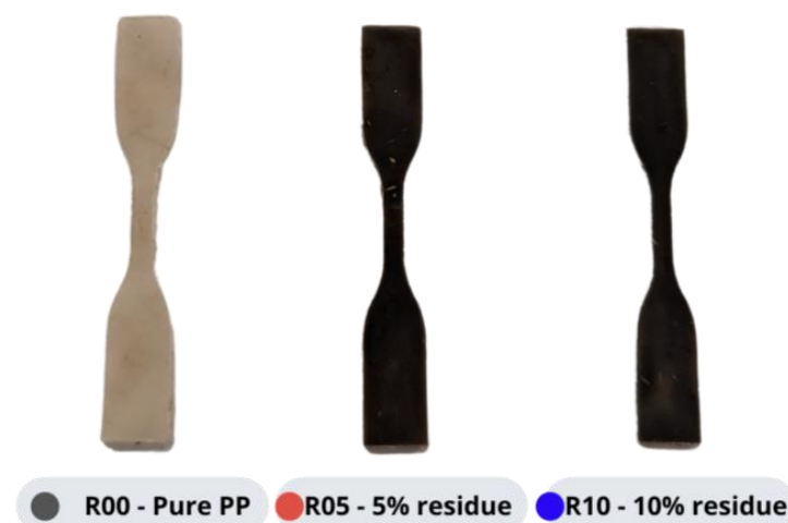
Figure 13. Specimens of the molded and pressed composite samples in butterfly shape.
