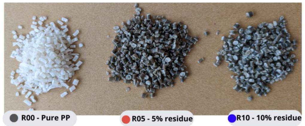
Figure 10. Pellets obtained after extrusion and pelletization of materials R00 (PP), R05 (PP + 5% Fluff), and R10 (PP + 10% Fluff) (% wt.).
