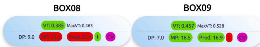
Fig. 5. Web platform developed. Visualization of the web platform interface developed for real-time monitoring and prediction of mechanical power (MP). Displayed are two patient monitoring boxes, BOX08 and BOX09, showing current tidal volume (VT), maximum VT, driving pressure (DP), current MP, and predicted MP. Alerts are indicated by red lights to signify when predicted values exceed threshold levels, and a 'CV' icon is present to indicate controlled ventilation status.
