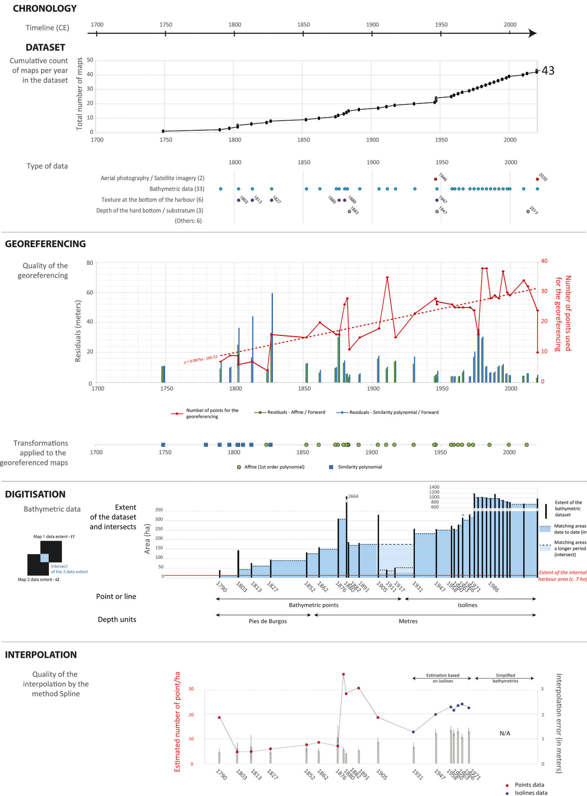
Fig. 2. Dataset of old maps and their characteristics, including a quality assessment of the georeferencing of the maps, the digitising, and the interpolation of the bathymetric data. All data are plotted referring to the date of the map.
