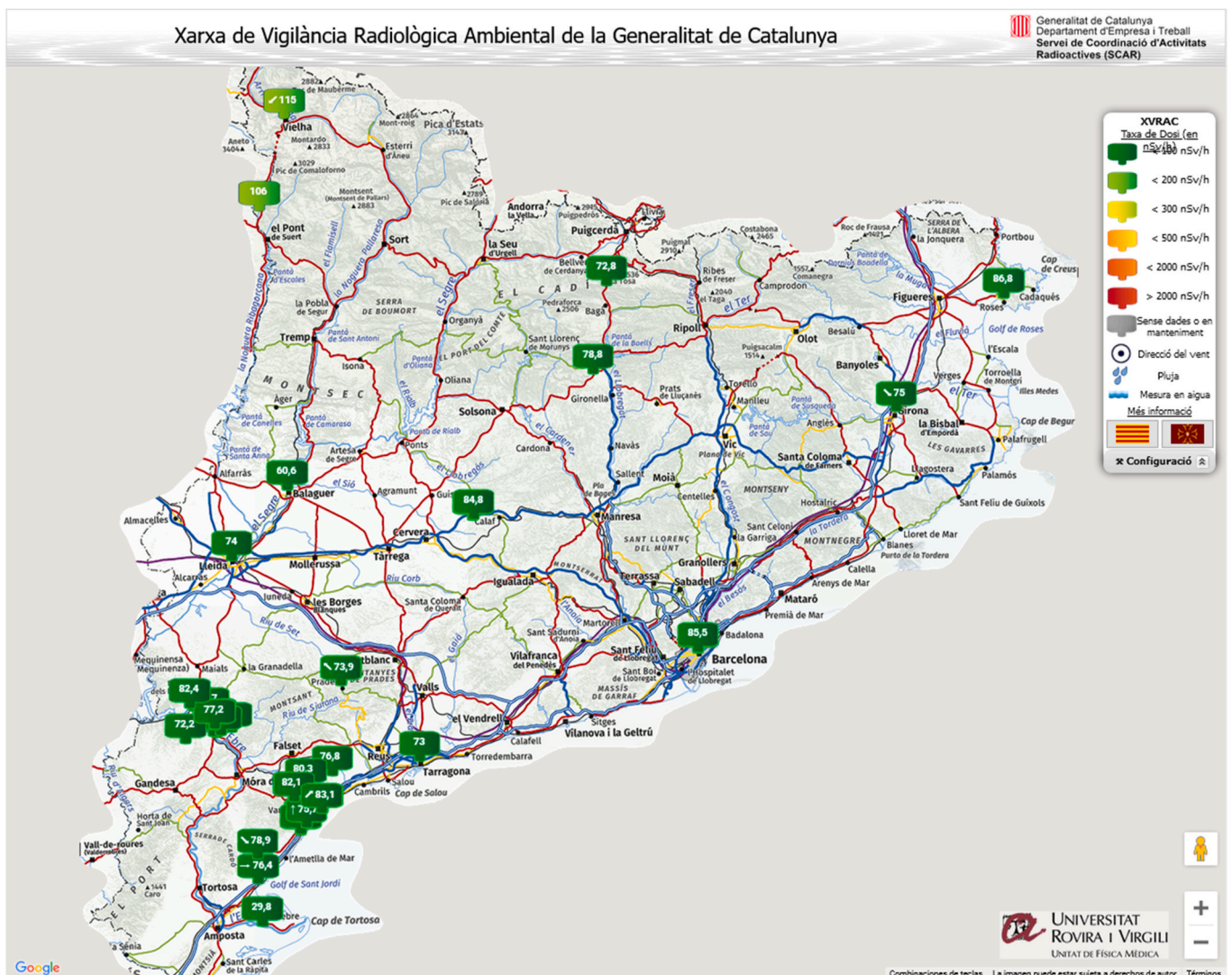
Fig. 1. General overview of XVRAC. All the monitors are showed with a green indication. The values presented show the dose rate (nSv/h) ( http://xvrac.fmurv.cat/ ).
