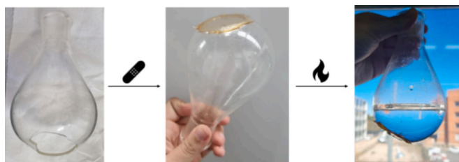
Fig. 7. Reparation of a broken flask with J100.
