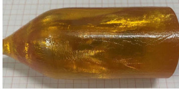
Fig. 1. A photograph of the as-grown Yb:Ca(Gd,Y)AlO 4 crystal boule, the growth direction is along the [001] axis.
