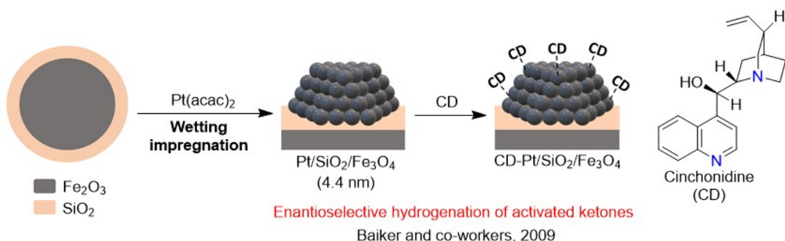
Fig. 12. Modification of Pt catalysts on silica coated Fe 3 O 4 by cinchonidine.
