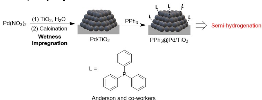
Fig. 21. Preparation and modification of a Pd/TiO 2 catalyst for application in the semi-hydrogenation of acetylene.
