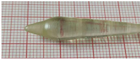
Fig. 1. Photograph of an as-grown 2.86 at.% Ho:YGG crystal (starting composition).
