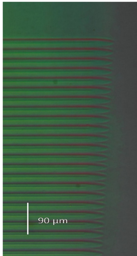
Figure 8. INTERPHAKO microphoto of a corner of the sinusoidal grating GL2, implanted in Er: Fe: LiNbO 3 by 5 MeV N 3+ ions. F = 5 \times 10^{15} ion/cm 2 . \Lambda = 16 μm.
