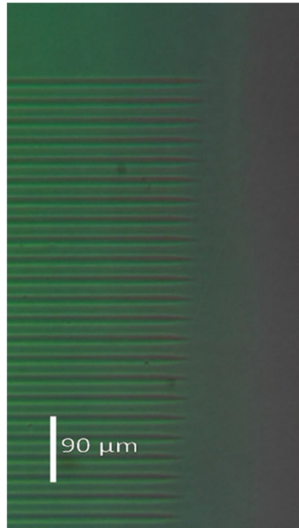
Figure 7. INTERPHAKO microphoto of a corner of the sinusoidal grating GL4, implanted in Er: Fe: LiNbO 3 by 10.5 MeV N 4+ ions. F = 1.4 \times 10^{15} ion/cm 2 . \Lambda = 16 μm.
