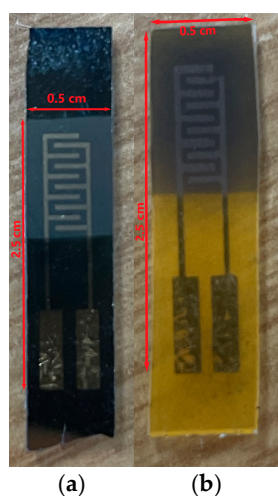
Figure 1. Pictures of the prepared sensors on the (a) silicon substrate and (b) Kapton substrate.
