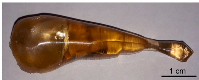
Fig. 1. A photograph showing an as-grown 0.2 at. % Yb 3+ -doped MgMoO 4 crystal (actual doping). The growth direction is along the [001] axis.
