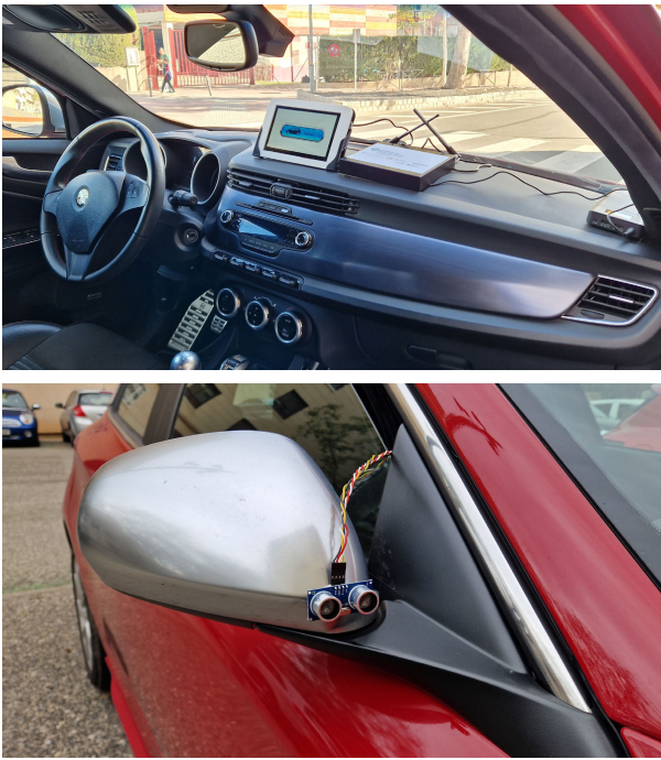
Fig. 6. In-vehicle set up (top). Detection ultrasonic sensor (bottom).
