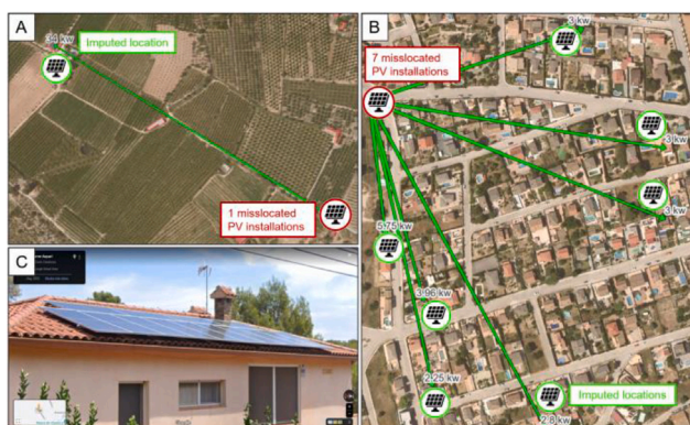
Fig. 5. Editing of approximate locations of solar PV installations in the province of Tarragona: (A) Most probable location, (B) Multiple PV locations geocoded at the electrical substation coordinates, and (C) Validation using Google Street View imagery, when available.
