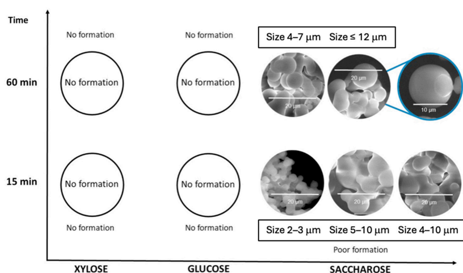
Figure 1. ESEM images of the carbon microspheres obtained by microwave-assisted hydrothermal treatment of 1.6 M aqueous solutions of commercial xylose, glucose, and saccharose at 180 °C under magnetic stirring for 15 and 60 min.
