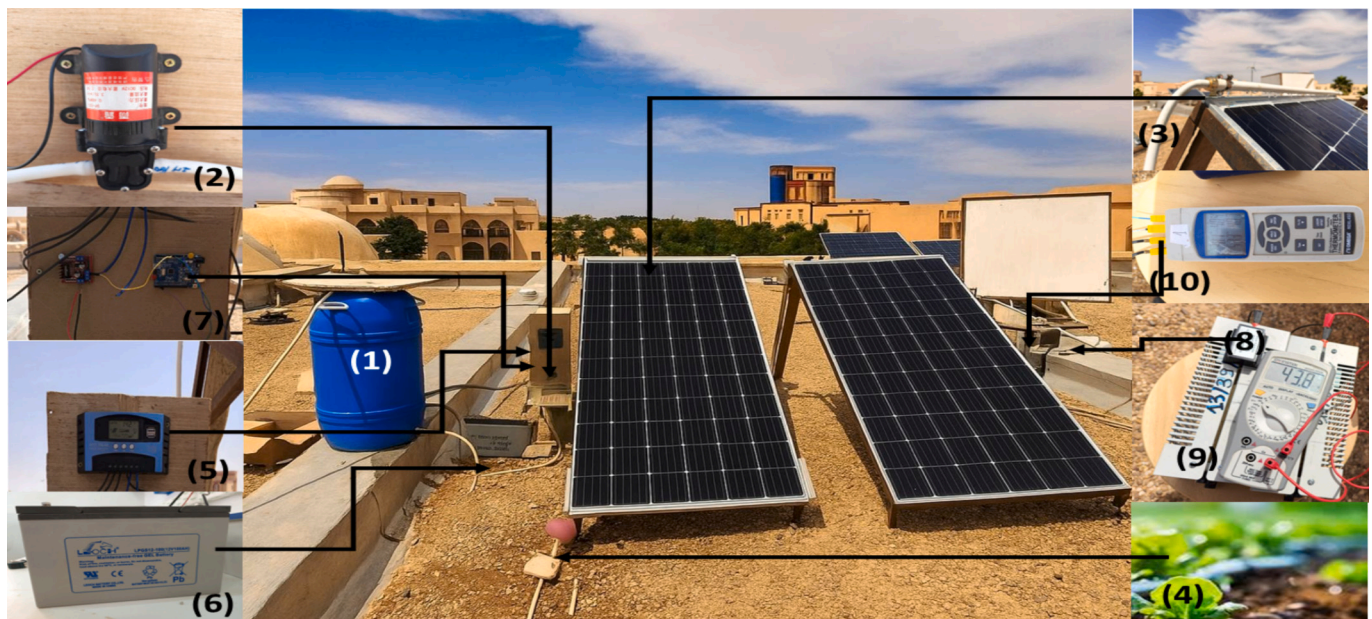
Fig. 4. Schematic Diagram of the PV Panel Cooling System. (A) PVT panel, (B) PV panel, (1) water tank, (2) pump, (3) Pipe outlets, (4) Green Space and Grass, (5) Solar charge controller, (6) Battery, (7) Arduino with Relay, (8) Rheostat, (9) multimeter, (10) thermometer. (For interpretation of the references to colour in this figure legend, the reader is referred to the web version of this article.)
