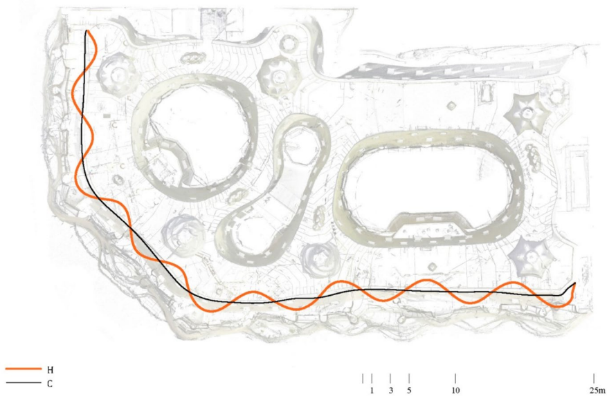
Fig. 10 Simple harmonic pulse representative of H = 7.961 \approx 8 cycles around the cornice. Figure created by the authors
