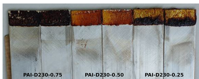
Figure 8. PAI adhesives after debonding at 160 °C, applying a 0.59 N constant force.
