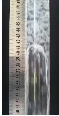
Figure. 3. A photo of slug regime obtained for U_{ls}=0.58 m/s and U_{gs}=0.23 m/s.
