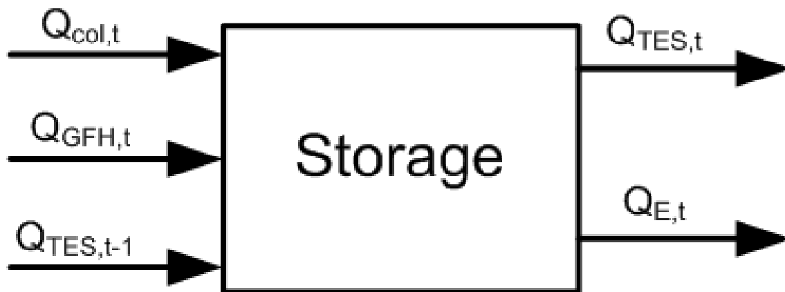
Figure 3: Energy balance applied to the storage system
